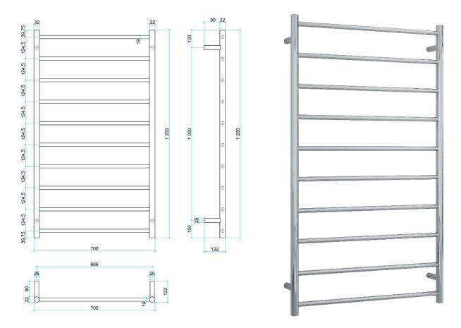
This rail has Multiflex wiring which means that there is a connection point on both the left and right hand side of the rail and the lead can be connected to either side. Being a dry electric element rail, this can be mounted either way up meaning the wiring can be from any of the four mounting points.
